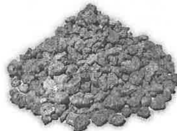
FIG. 3 STEEL SLAG AGGREGATE
