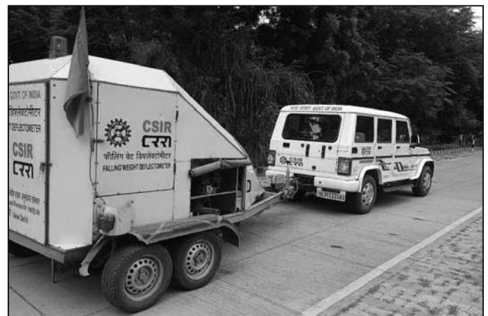
Fig.1 Field Testing Set for Falling Weight Deflectometer (FWD) Measurement
