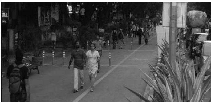
Photo 39 Mock Trial Run of Urban Street Project using Temporary Elements like Plastic Bollards
